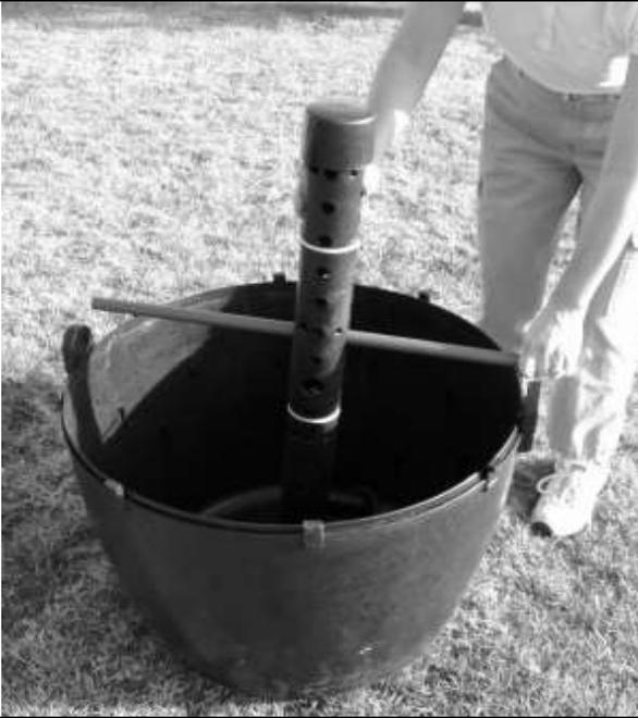
Check and be sure the aeration tube has been snapped together, secured with two Ty-Wraps (shown as white here but are usually black), the cap is snugged down and the breaker bar inserted.
