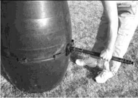
If you have not put the aeration tube assembly into the barrel yet, do it now. Press the Pivot Rod through the barrel halves and through the Aeration Tube. It should look like the picture on the right here. (Except for the optional breaker bar which most people will not have.)
