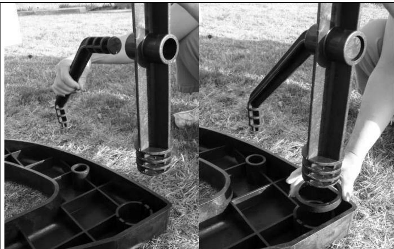
Lay one of the stand halves flat on the ground. Insert a Gusset Brace into a Stand Support. Place a Retainer Ring (large opening side down) over the end of the Support Bar, pressing the Support Bar and Gusset Brace into the stand. Be sure the Gusset Brace and Support Bar is pressed all the way into their sockets. **NOTE: Usually the Retainer Rings are not loose in the box but pressed onto the Stand Halves already.**
