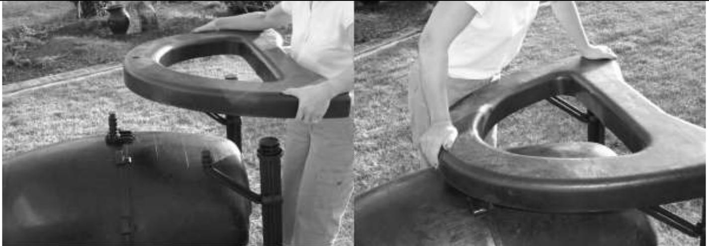
Align the second Stand Half with the Pivot Rod, both Gusset Braces, and both Stand Supports. At first, gently align all of these parts with the appropriate holes being careful not to damage the Retainer Rings. Just let the Stand Half rest in place. Then by hand, press the Retainer Rings up into place over the Stand sockets. Now firmly press down on the Stand making sure all of the components are inserted with their locks fully engaged.
