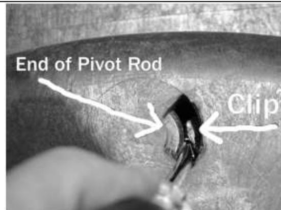
To the right here is looking down from the top of the stand. While holding the clip away from the pivot rod to allow it to slide out, insert a second flat head screwdriver between the stand and barrel and begin prying the barrel away from the stand.
