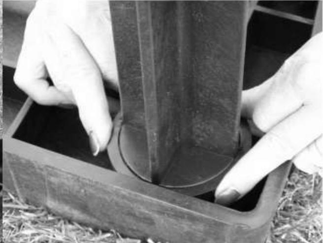
Insert the same assembly on the other side of the stand. Make sure the locks in the Stand are fully engaged in the Stand Supports. Then check to see the Retainer Ring is securely seated. There is a ridge or bump on the Stand Support itself that should be helping to lock this ring in place.
