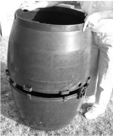
The barrel halves use a tongue & groove connection. Review the next page before continuing. Be sure to liberally coat both sides of the tongue on the bottom half of the barrel with vegetable oil (or similar lubricant) before attempting to put the halves together. Also put some oil on the surfaces of the locks where they come together.
