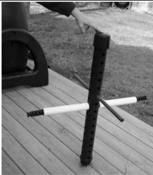
As an option, we have added two 11" PVC sleeves over the pivot rod as shown here to help prevent ovaling of the barrel when holding extra heavy loads.
